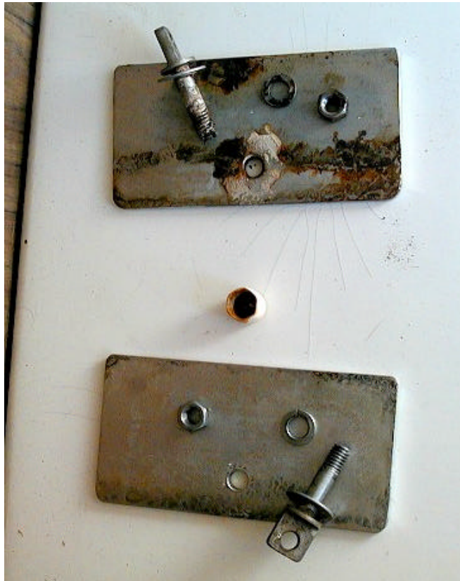
Figure 2 Old eyebolt backing plates. Starboard aft plate top, starboard forward plate bottom.
