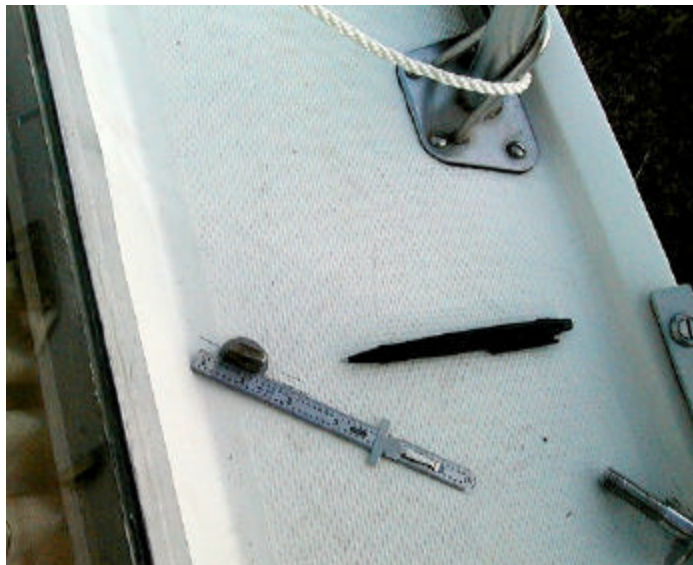
Figure 4 Marking the orientation of the old eyebolts prior to removal.
