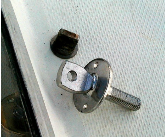
Figure 1 Old vs. New. The new eyebolt has a much larger flange, a larger cross section, and two screw holes to prevent eyebolt rotation.
